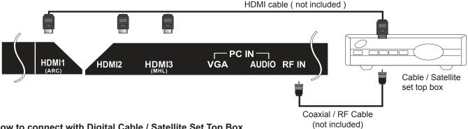
How to connect with Digital Cable / Satellite Set Top Box
