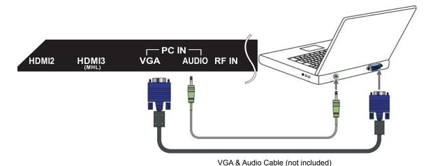
Recommended computer display resolution:1366x768@60 Hz
