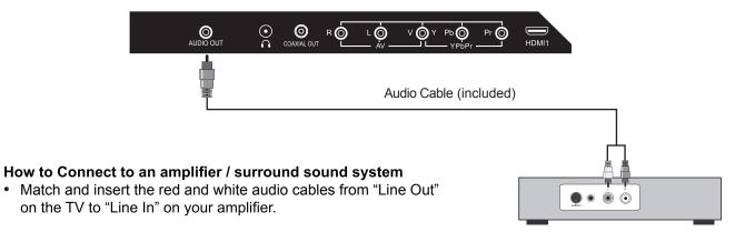
NOTE: The TV's speakers will still output audio. You can turn the TV's speaker volume to 0 to prevent echoing.
