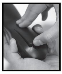
• Turn the remote over and remove battery cover.
