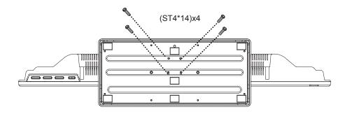
Insert 4 screws (provided) through the holes in the bottom of the base into the post holes and tighten securely. Do not over-tighten.
