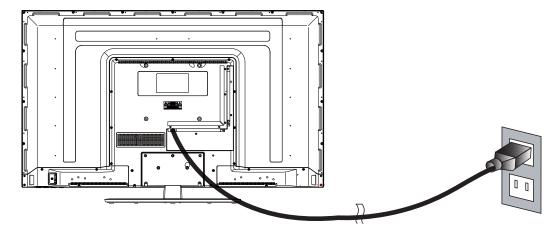
• Connect the power cord to a properly grounded AC outlet.
