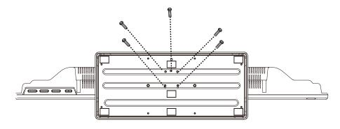
Insert 5 screws (provided) through the holes in the bottom of the base into the post holes and tighten securely. Do not over-tighten.
