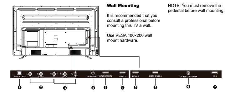
**1. OPTICAL OUT** - Connect to an AV Receiver for high quality digital audio.
