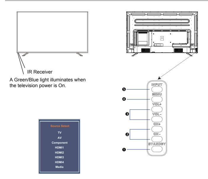
1. **STANDBY/POWER** - Press the **STANDBY** button to turn the TV ON/ OFF (power). The screen image will appear within a few seconds, and the LED will turn on.
