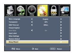
• Setup Wizard Set the first time installation. Press ENTER / ► button to enter.
