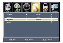
• Press down ▼ arrow button to highlight **Digital CC**. Navigate using the ◀ ▶ arrow buttons to select **Off**, **Service 1-6**.
