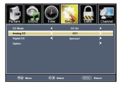
Press down ▼ arrow button to highlight Analog CC. Navigate using the ◀ ▶ arrow buttons to select CC1-4, TEXT1-4.
