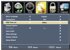
• **OSD Time Out** Adjust the duration of the OSD (on screen display) menu. Press ◀ ▶ button to select.
