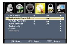
Press the down ▼ arrow button to highlight Device Auto Power Off. Navigate using the ◀ ▶ arrow buttons to select On - Off.
