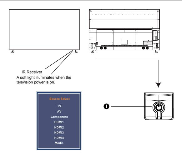
1. **POWER** - Press the **POWER** button to turn the TV ON/ OFF (power). The screen image will appear within a few seconds, and the LED will turn on.
