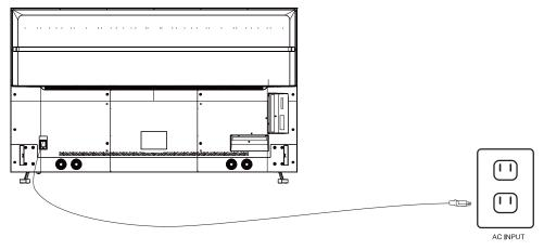
· Connect the power cord to a properly grounded AC outlet.
