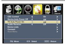
Press down ▼ arrow button to highlight TV Auto Power On. Navigate using the ◀ ▶ arrow buttons to select On - Off
