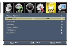
To make changes to parental controls, highlight System Lock then press the ◀ ▶ arrow button to ON.
