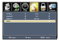
Press down ▼ arrow button to highlight Option. Press the ► arrow button to enter a menu with options to customize text fonts, colors and opacities.
