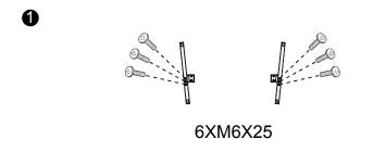
Insert 6 screws M6X25 (provided) through the holes in the bottom of the base into the post holes and tighten securely. Do not over-tighten.
