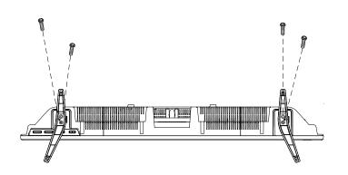
Insert 4 screws (provided) through the holes in the bottom of the base into the post holes and tighten securely. Do not over-tighten.
