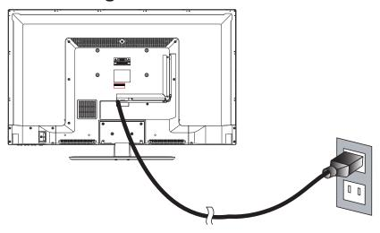
· Connect the power cord to a properly grounded AC outlet.
