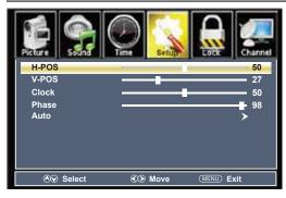
Highlight H-Pos. Navigate using the ◀ ▶ arrow buttons to adjust the position of images displayed from side to side.
