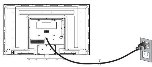
• Connect the power cord to a properly grounded AC outlet.
