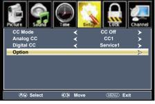
• Press down ▼ arrow button to highlight **Option**. Press the ▶ arrow button to enter a menu with options to customize text fonts, colors and opacities.
