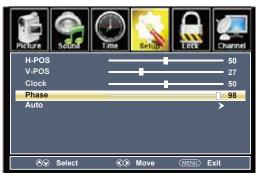
• Highlight **Phase**. Navigate using the ◀ ▶ arrow buttons to improve focus and image stability.
