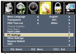
Gain access to position adjustment options by pressing the down ▼ arrow button to highlight PC Settings, then press ► arrow button to select from the following options.
