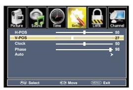
Highlight V-Pos. Navigate using the ◀ ▶ arrow buttons to adjust the position of images displayed up and down.
