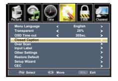
• Press the down ▼ arrow button to highlight Closed Caption then press the ▶ arrow button to highlight CC Mode.
