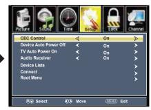
If this item is "On", users can control the volume of a compatible external amplifier through adjusting the TV's volume.
