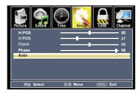
• Highlight **Auto**. Press the ► arrow button to automatically adjust the display to the best setting.
