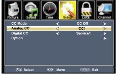
Press down ▼ arrow button to highlight Analog CC. Navigate using the ◀ ▶ arrow buttons to select CC1-4, TEXT1-4.
