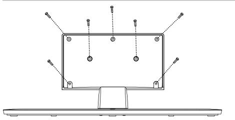
To use the TV with a wall mount first remove the base by removing the 7 screws shown to the left.
