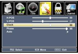
• Highlight **Clock**. Navigate using the ◀ ▶ arrow buttons to control the width of the image.
