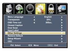
• Other Settings Adjust the settings for Audio Only, No Signal Power Off, and No Operation Power Off. Press ENTER / ▶ button to enter.
