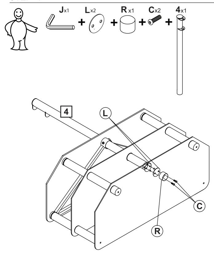
WARNING: ONLY USE A HAND SCREWDRIVER TO TIGHTEN ALL SCREWS DURING ASSEMBLY. DO NOT USE POWER SCREWDRIVER or RILL OF ANY KIND DURING ASSEMBLY.
