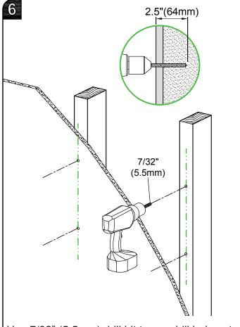
Use 7/32" (5.5mm) drill bit to pre-drill holes at least 2.5" inches (64mm) deep at the marked locations.
