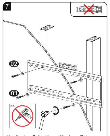
Use the Lag Bolts (1) and Washers (2) to secure the Wall Plate to the wall.
