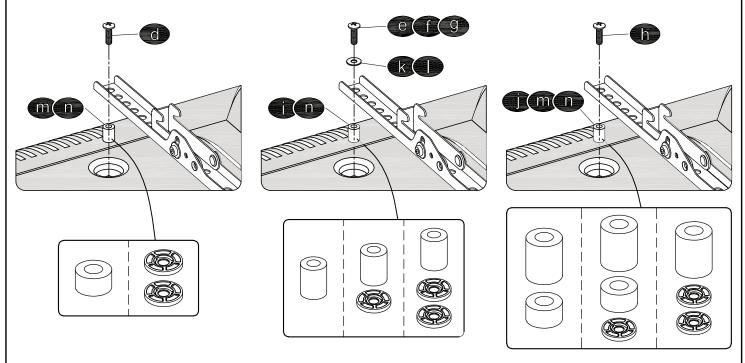
Tips: If you need to combine M8(d/h) screw with 2.5mm spacer(n), you have to remove the inner circle of Spacer (n).
