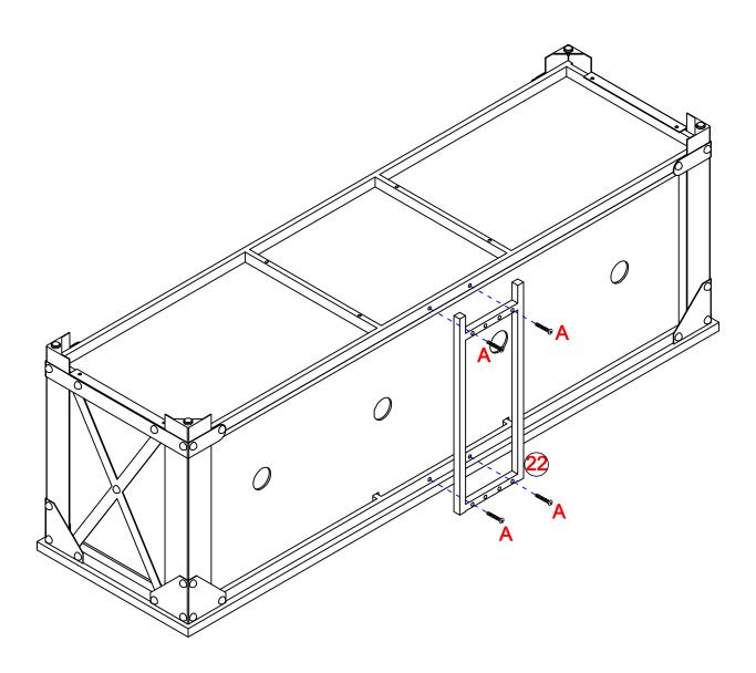
\* Please lift the iron frame, when turning over the cabinet Do not lift the wood top
