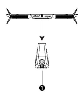
1. **POWER/STANDBY** - Press the **POWER** button to turn the TV ON/ OFF (power). The screen image will appear within a few seconds, and the LED will turn on.
