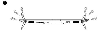
Insert 6 screws ST4X24 (provided) through the holes in the bottom of the base into the post holes and tighten securely. Do not over-tighten.
