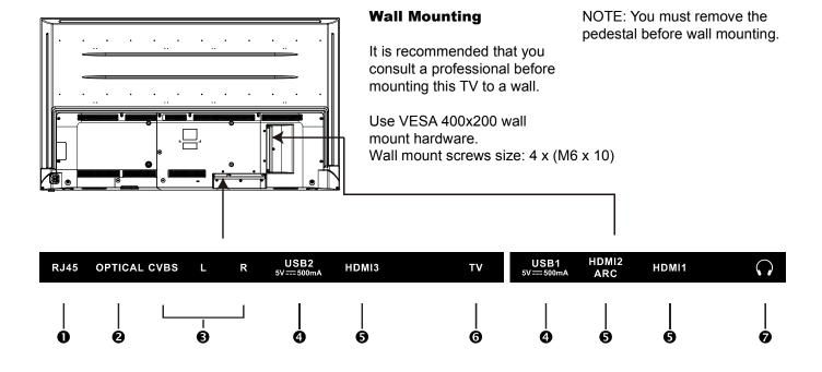
1. RJ45 - RJ45 plug for connecting to external modem or network access equipment.
